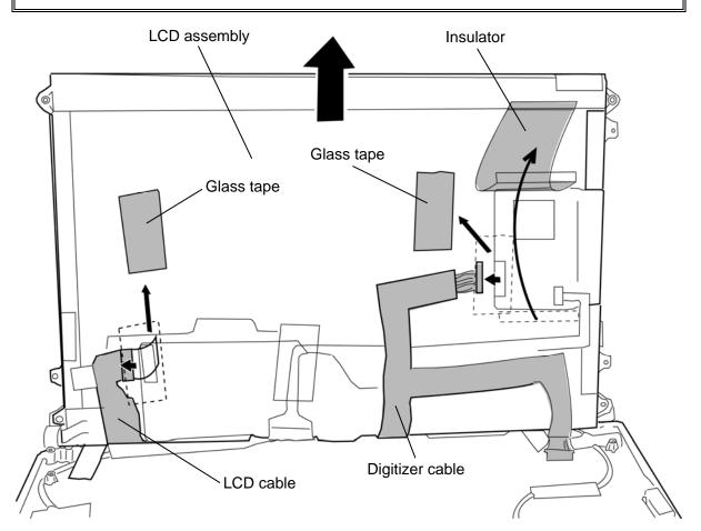
Figure 4-53 Removing the LCD assembly (2)
